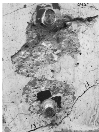
图11 锚栓位置处混凝土压碎现象 Fig.11 Concrete crushing near bolt shaft
