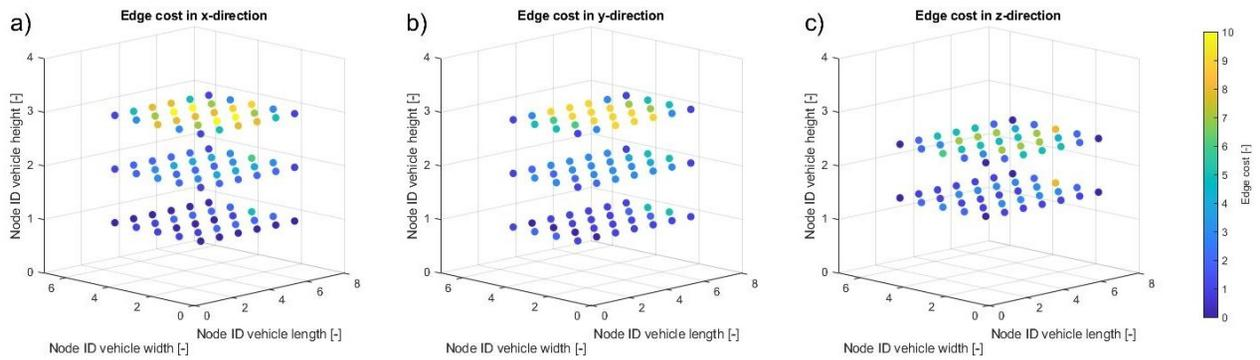
**Fig. 4 Edge cost of a vehicle wiring harness E-structure in a)  $x$ -direction, b)  $y$ -direction and c)  $z$ -direction dependent on the distance to preferred cable paths)**
