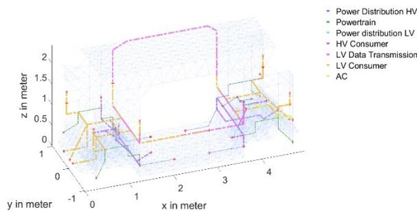
**Fig.7 Cable routing with the optimization tool in an automated electric vehicle (autoSHUTTLE)**
