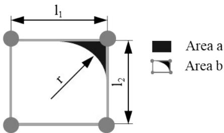
**Fig.5 Inaccuracies on bending radius  $r$  dependent on the area of a grid element ( $l_1 \cdot l_2$ )**
