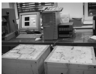
图1 普通混凝土和PCM混凝土的温度监测 Fig.1 Temperature measurement of concrete and PCM concrete
