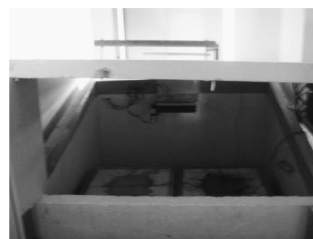
图2 大体积混凝土内部热环境模拟房 Fig.2 Chamber simulating temperature condition of mass concrete
