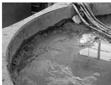
图6 EL4 工况后的冒砂现象 Fig.6 Sand boiling phenomenon after the excitation of EL4
