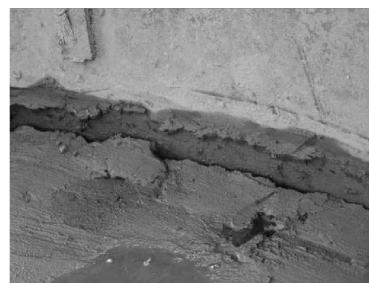
图7 试验后土体的下沉情况 Fig.7 Subsidence of the soil after the test
