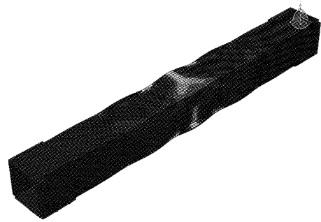
图 21 试件在最大承载力时刻对应的塑性应变发展情况 Fig.21 Distribution of plastic strain when reaching bearing capacity
