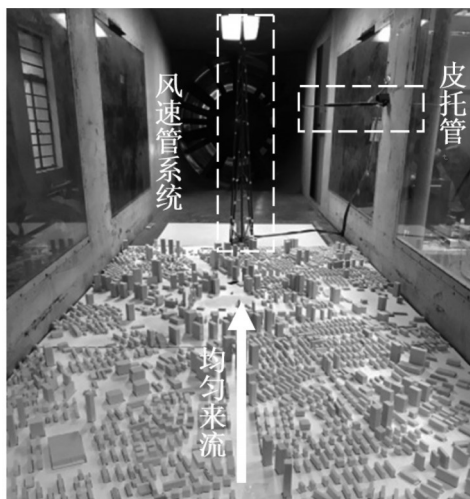
图2 试验部分测量设备及模型的布置 Fig. 2 The arrangement of equipments and models
