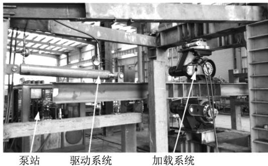
Fig. 5 Actual image of wear test-bed
