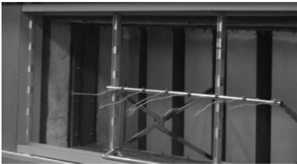
图9 缓冲口丝带法测量 Fig.9 Wire test of buffer region
