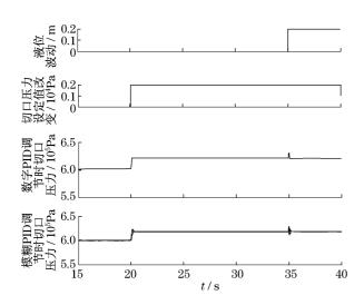
图 3 跟随输入阶跃变化和存在阶跃扰动时的输出响应 Fig. 3 Output response following the step change of the input and the disturbance
