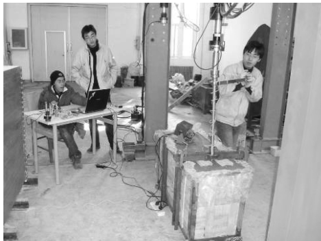
图 7 模型钻头钻入水泥土介质试验照片 Fig. 7 Photo of model auger drilling into cement-soil mixture
