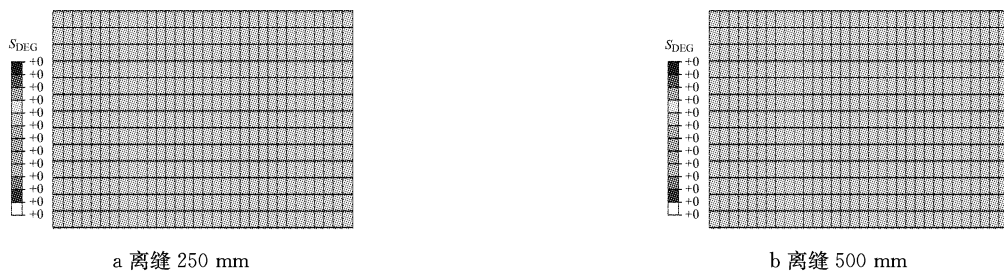
图 8 顶推压力 0.8 MPa 条件下的刚度下降率 Fig.8 Stiffness reduction rate of a 0.8 MPa pushing pressure
