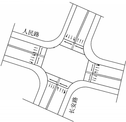
图3 交叉口交通设计图 Fig. 3 Layout of intersection and signal groups
