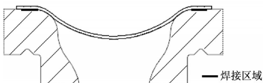
图3 焊接后爆破片区域截面示意 Fig. 3 Section view of burst disk after welding
