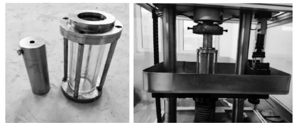
图 6 气泡基壁后注浆材料压缩特性试验磨具及压缩过程 Fig. 6 Test tool and compression process for compression characteristics of foam base wall backfill material
